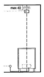
NOTE! The thermostat is located above the sauna heater
