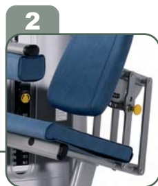
靠背與座椅保持100° Back Pad is Angled 100° from Seat Bottom
