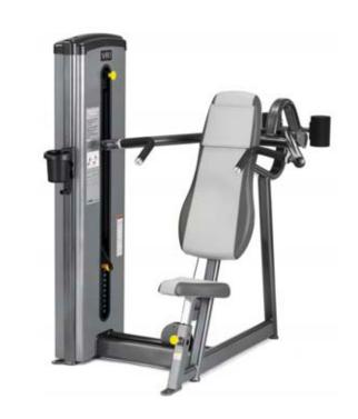
Counterbalanced input provides reduced takeoff weight for deconditioned users.
