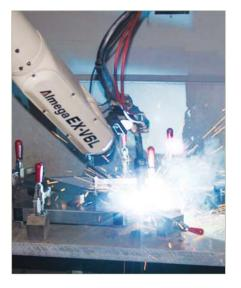
Top: Coordinate Measurement Machine (CMM) Above: Pulse Robot Welder Right: Sheet Laser
